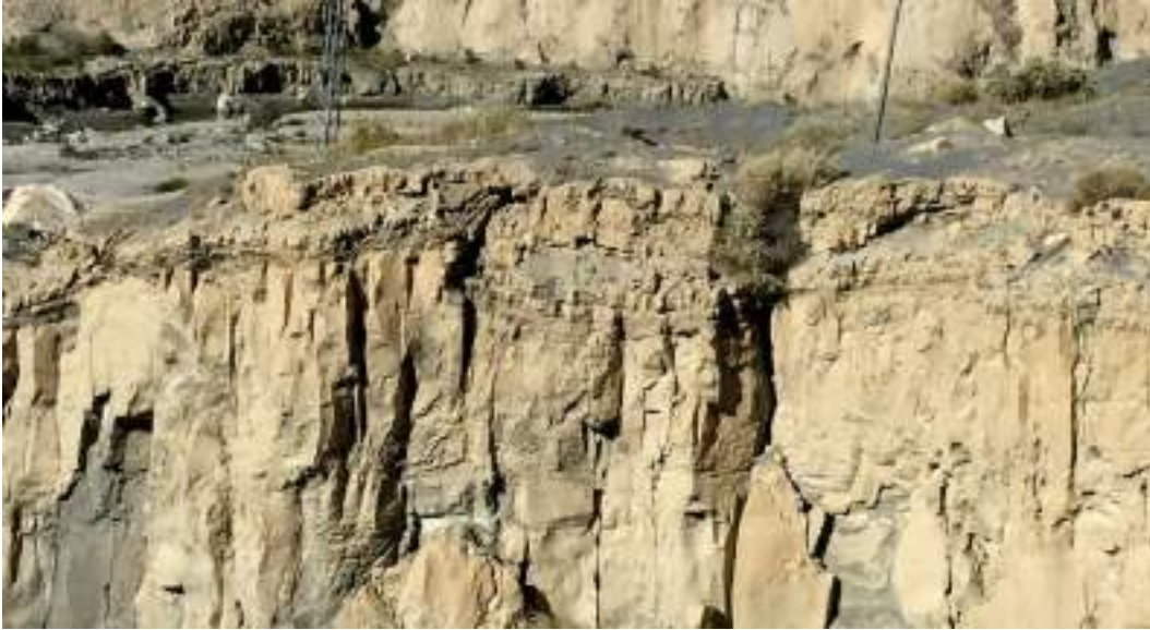
Photo 6-17 Micro thrust fault in clayey silt beds near helipad.
