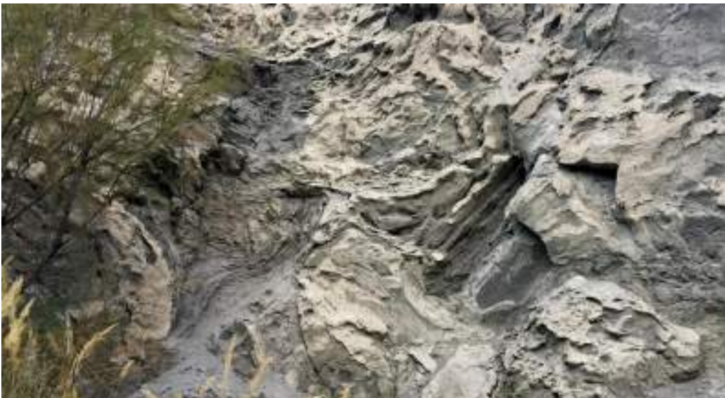
Photo 6-13 Sheared and Smeared Clayey Silt at Sarat Village.
