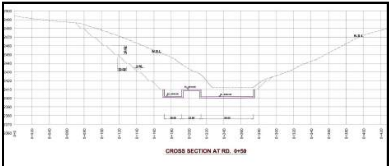
Figure 10-1: Cross Section at Chainage 0+50
