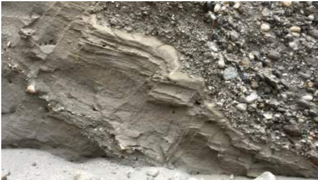
Photo 6-23 Development of Micro Faults in Sand.
